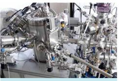
*The electron spectrometer at EMSL is* used to study the chemical properties of materials at nanoscale resolution.
