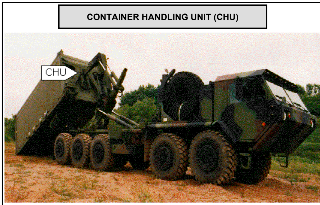
Figure J-7. Container Handling Unit (CHU)
