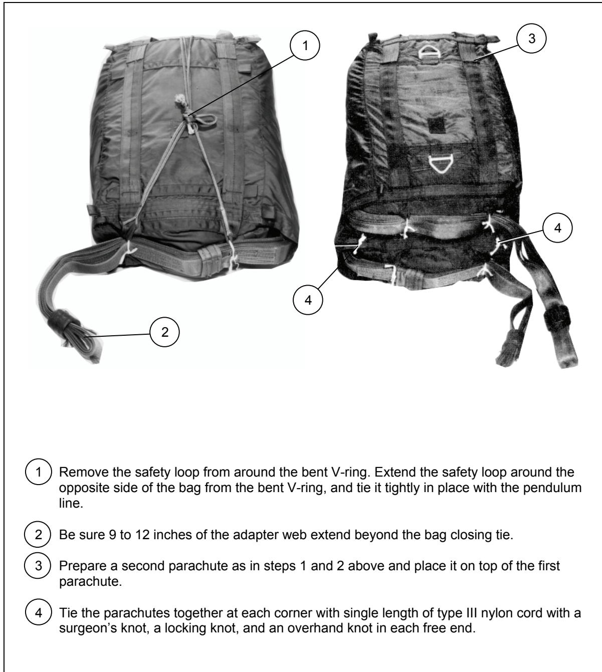
Figure 9-7. Clustering Extraction Parachutes for a Sequential Extraction
