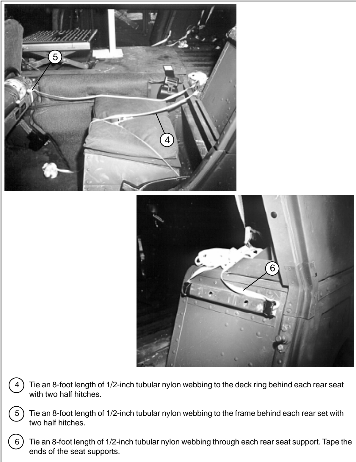
Figure 5-2. G/VLLD and Accompanying Equipment Rigged in M966 Truck (continued)
