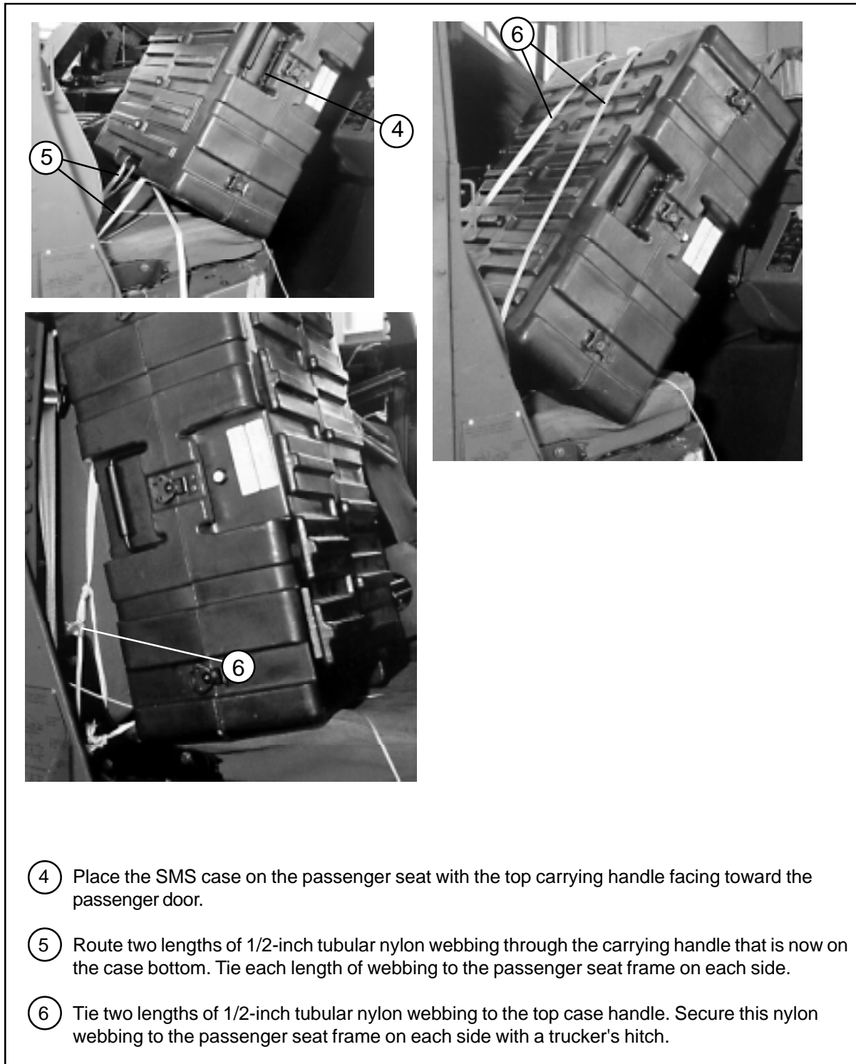
Figure 5-11. Rigging SMS in Cargo/Troop Carrier (continued)
