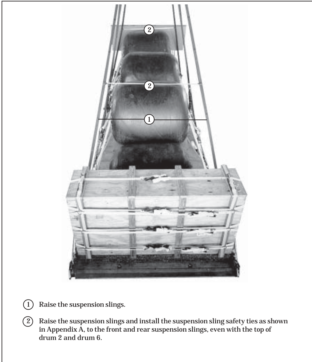
Figure 1-63. Suspension Slings Safety Tied
