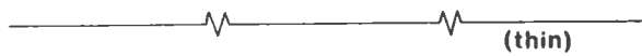
Figure 14-10 How to draw breaklines. The wavy line used for shorter breaks is drawn freehand whereas the line for longer breaks is drawn as shown.
