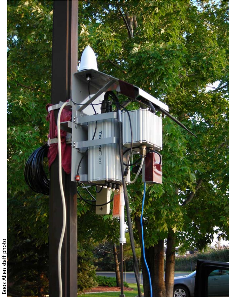
Figure 2-17: RSE Assembly Mounted on Pole for Test
