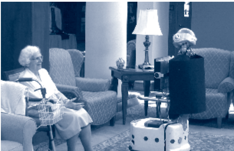
A participant in an NINR-funded study meets "Pearl," a humanoid from the Nursebot Project, in which nurse scientists aimed to learn how older adults would respond to navigational guidance offered by a mobile robot.
