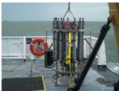
Figure 1. Water sampling package on stern of Thomas Jefferson
