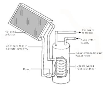
Active, indirect systems are often used in climates with freezing temperatures.
