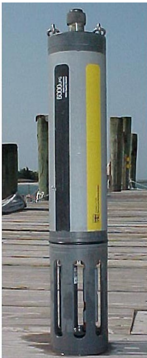
This is a YSI 6000 UPG Multi-Parameter Water Quality Monitor. This particular model measures dissolved oxygen, salinity, temperature, pH, depth, and turbidity. Click on image for more details. (Photo: North Carolina NERRS site)
