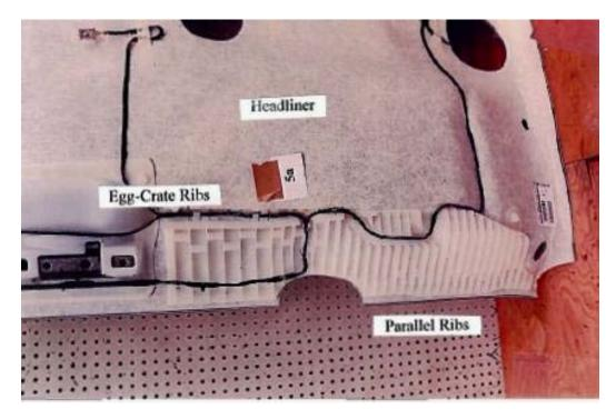
Figure 1: Egg-Crate and Parallel Ribs Built into the Headliner<sup>8</sup>
