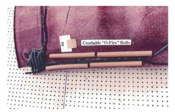
Figure 4: Crushable O-Flex Rolls<sup>9</sup>
