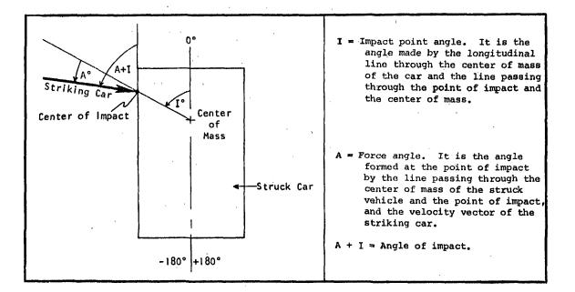
Figure 3-1. Diagram for measuring "Impact Point" and "Force" angles.
