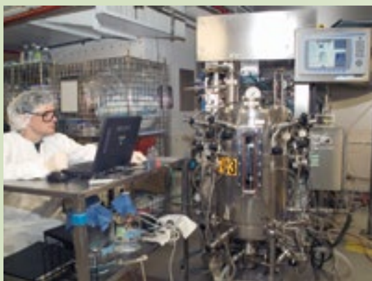
cGMP 80L Fermentation of rhIL-15. Production of rhIL-15 involves refolding, purification, and pooling of product derived from fermentation paste. Several fermentations in this 80-L fermentor at 50-L working volume are run for one 1-gram lot of rhIL-15.
