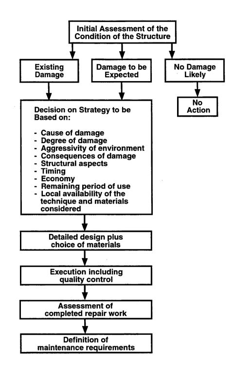
Fig. 3.4 Steps to be taken in a repair process. Source: Technical Committee 124-SRC, "Draft Recommendation for Repair Strategies for Concrete Structures Damaged by Reinforcement Corrosion," pp. 415-436 in *Materials and Structures* 27(171), International Union of Testing and Research Laboratories for Materials and Structures (RILEM), Cachan, France; adapted with permission from RILEM.
