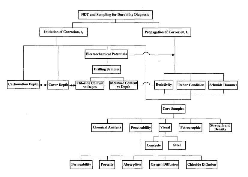
Fig. 3.1 Techniques for assessing deterioration. Source: R. D. Browne, "Durability of Reinforced Concrete Structures," *Pacific Concrete Conference*, Proceedings Vol. 3, Auckland, New Zealand, New Zealand Concrete Society, November 1988; reprinted with permission from author.
