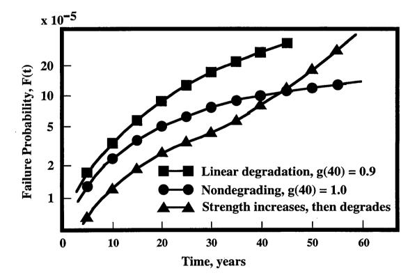
Fig. 5.3 Failure probability of a one-way slab.
