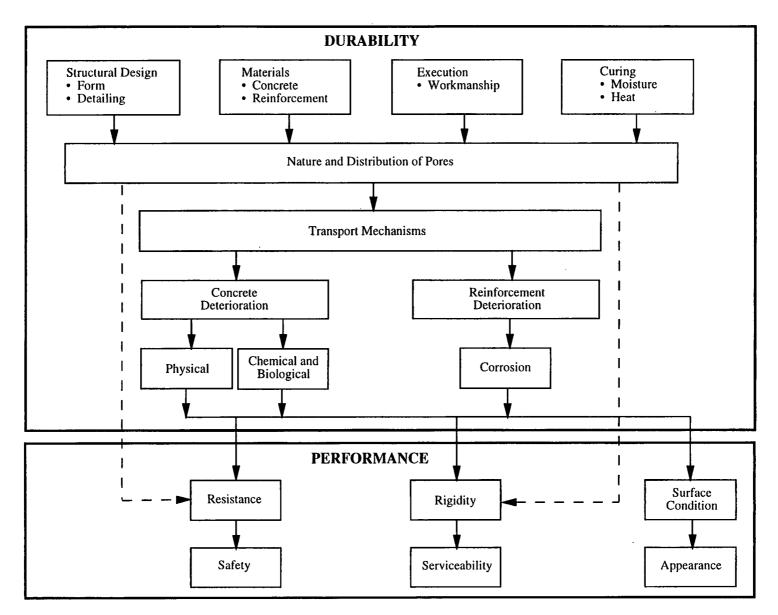
Fig. 2.8 Relationship between the concepts of concrete durability and performance. Source: Comité Euro-International du Béton (CEB), *Durable Concrete Structures–Design Guide*, published by Thomas Telford Services Ltd., London, England, 1989; reprinted with permission from CEB and Thomas Telford Services Ltd.
