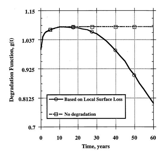
Fig. 5.8 Mean degradation function of wall in flexure/compression.
