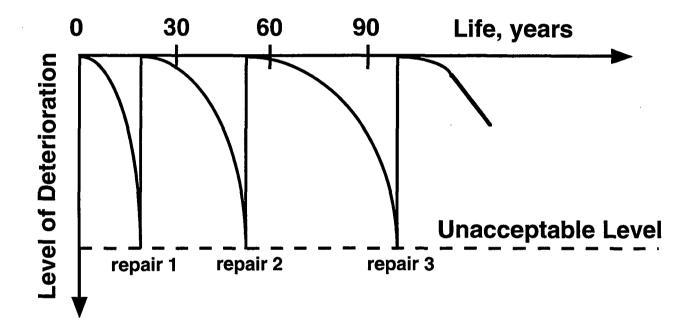
Fig. 3.3 Effect of multiple repairs over the life of a structure.
