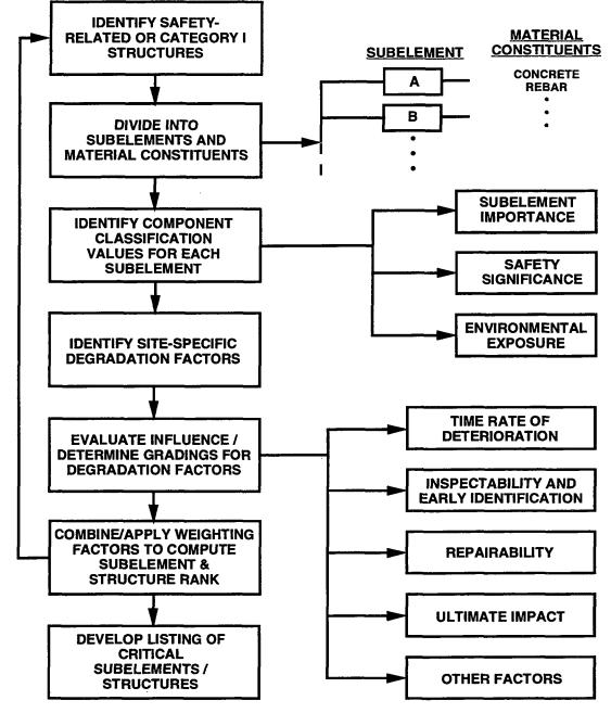
Fig. 4.1. Structural aging assessment methodology flow diagram.
