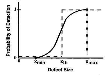
Fig. 5.10 Probability of detection of a defect of size x.
