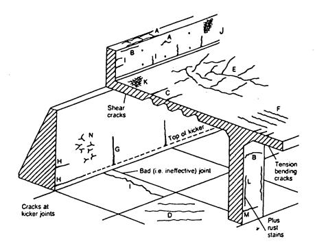
A = plastic settlement, over reinforcement B = plastic settlement, arching C = plastic settlement, change of depth D = plastic shrinkage, diagonal E = plastic shrinkage, random F = plastic shrinkage, over reinforcement G = early thermal contraction, external restraint H = early thermal contraction, internal restraint I = long-term drying shrinkage J = crazing, against formwork K = crazing, floated concrete L = corrosion of steel reinforcement
