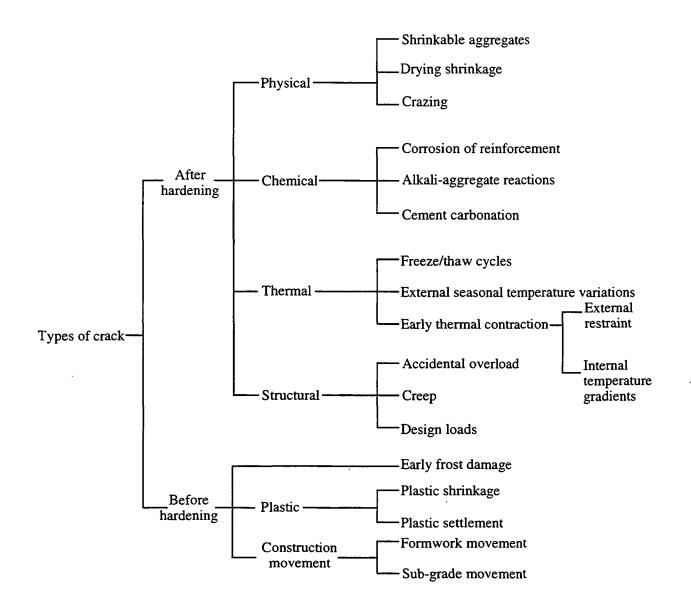
Fig. 2.9 Relationship between primary causes and types of cracks that can occur in concrete. Source: Comité Euro-International du Béton (CEB), *Durable Concrete Structures–Design Guide*, published by Thomas Telford Services Ltd., London, England, 1989; reprinted with permission from CEB and Thomas Telford Services Ltd.
