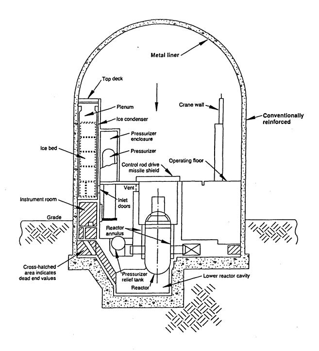
Fig. 2.5 PWR reinforced concrete containment with ice condenser.
