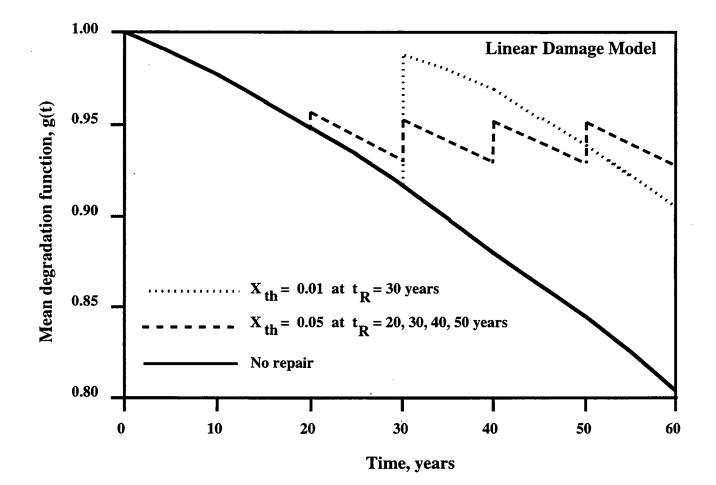
Fig. 5.12 Effect of multiple inspection/repairs on mean degradation function.
