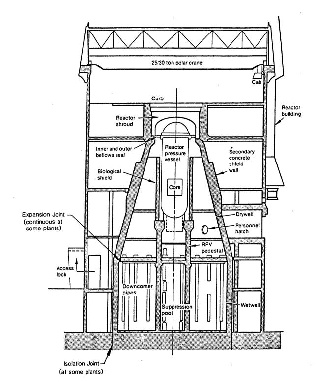
Fig. 2.2 BWR Mark II type reinforced concrete containment. Source: Copyright © 1994. Electric Power Research Institute. EPRI TR-103840-R1. BWR Containments License Renewal Industry Report: Revision 1. Reprinted with Permission.
