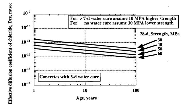
Fig. 2.16 Effective diffusion coefficient of chloride versus time for ordinary portland cement concretes.<sup>123</sup>
