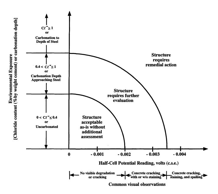
Fig. 4.3 Damage state chart relating environmental exposure, half-cell potential reading, and necessity for additional evaluation or repair
