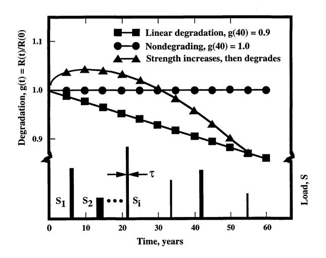
Fig. 5.2 Mean degradation functions of one-way slab.
