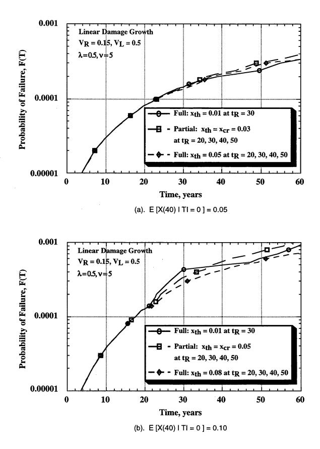
Fig. 5.14 Failure probability of a component with partial inspection.
