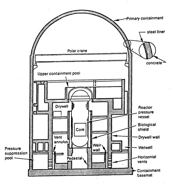
Fig. 2.3 BWR Mark III type reinforced concrete containment. Source: Copyright © 1994. Electric Power Research Institute. EPRI TR-103840-R1. BWR Containments License Renewal Industry Report: Revision 1. Reprinted with Permission.
