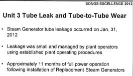
Inspections found unexpected Tube-to-Tube Wear
