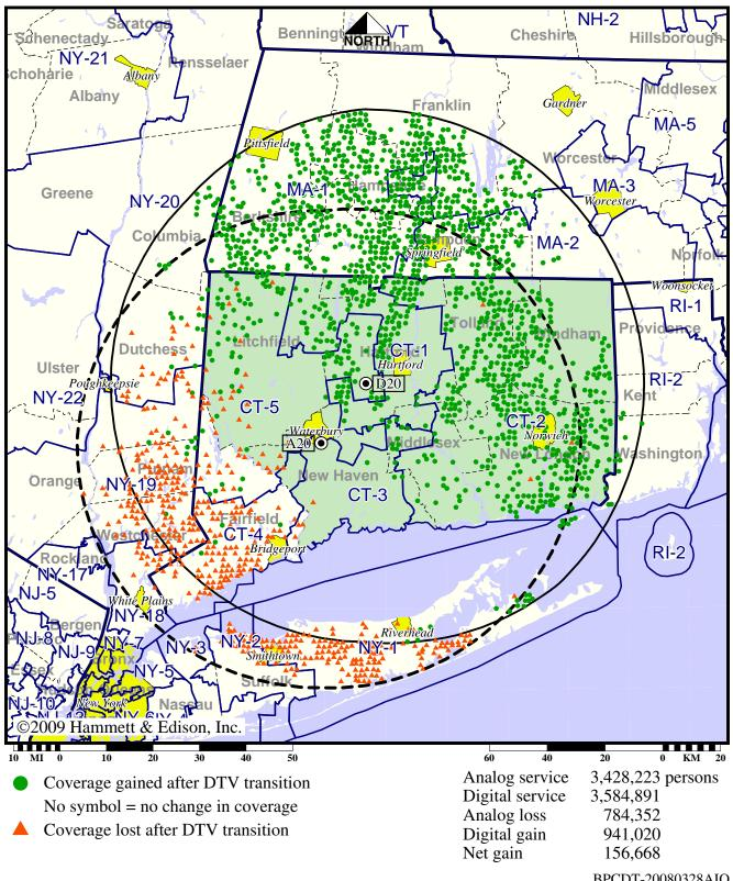
Digital CP (solid): 52.0 kW ERP at 516 m HAAT vs. Analog (dashed): 2240 kW ERP at 366 m HAAT
