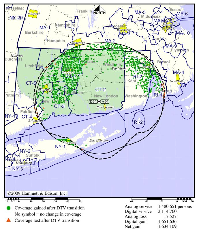
Digital CP (solid): 475 kW ERP at 384 m HAAT vs. Analog (dashed): 2820 kW ERP at 381 m HAAT
