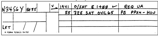
FIG 4-2-5 Flight Progress Strip
