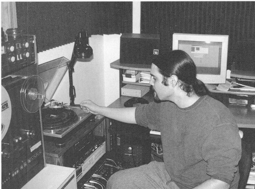
At the Cutting Corporation, in Bethesda, Maryland, sound preservation engineer Ryan Davis makes a digital transfer of an analog glass-based disc recording from the Eloise Hubbard Linscott Collection to create a digital file. Photo by James Hardin
