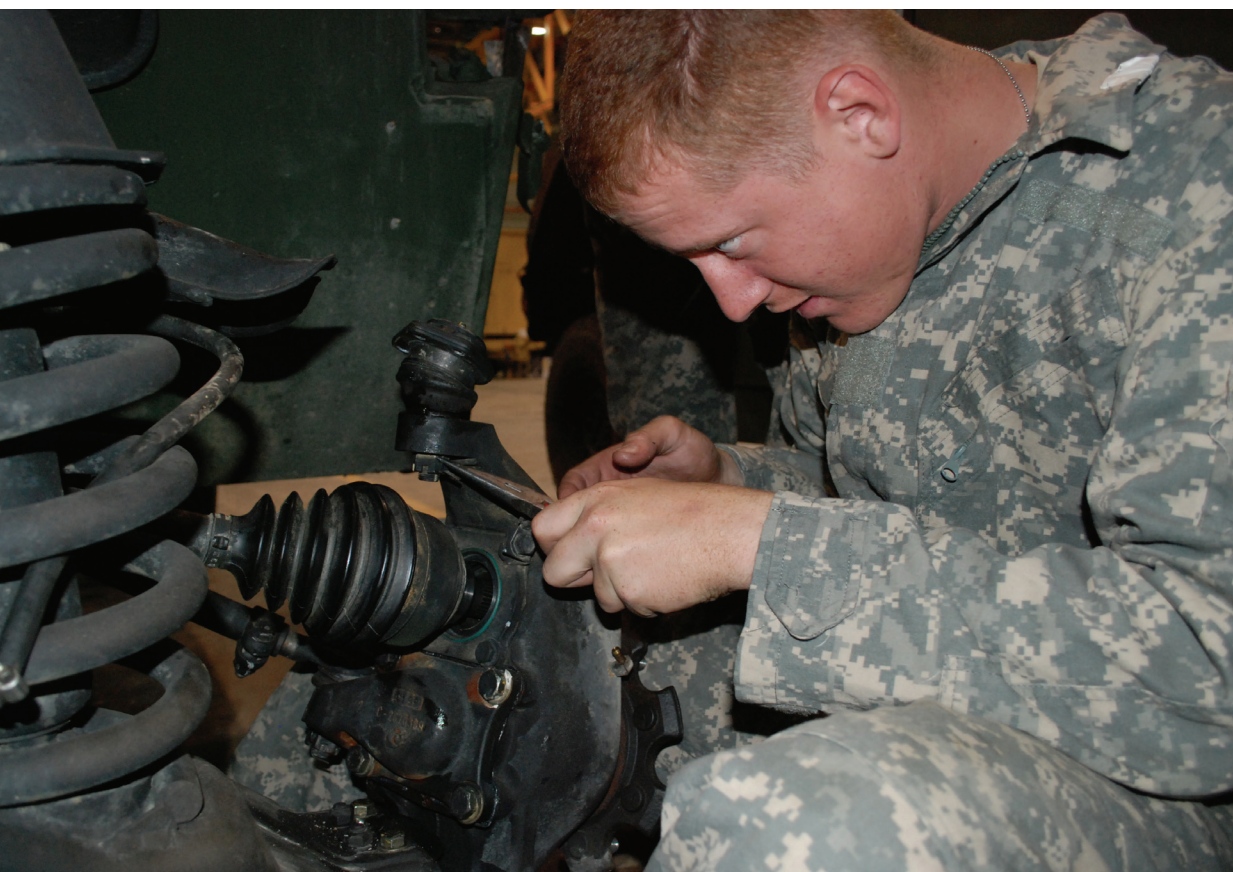
A wheeled-vehicle mechanic with the 1st Maintenance Company, 541st Combat Sustainment Support Battalion, from Fort Riley, Kansas, replaces an upper ball joint on a high-mobility multipurpose wheeled vehicle during a tasking to inspect and service military vehicles for the 1st Stryker Brigade Combat Team, 25th Infantry Division, at Fort Wainwright, Alaska. (Photo by SSG Trish McMurphy, U.S. Army Alaska PAO)
