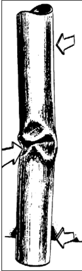
Figure D-7. Bending load failure
