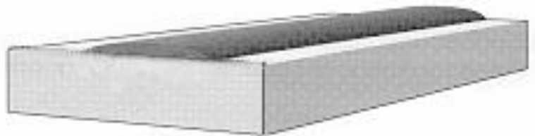
Figure 15. Material Fused to a Surface Using the Laser Bonding Process
