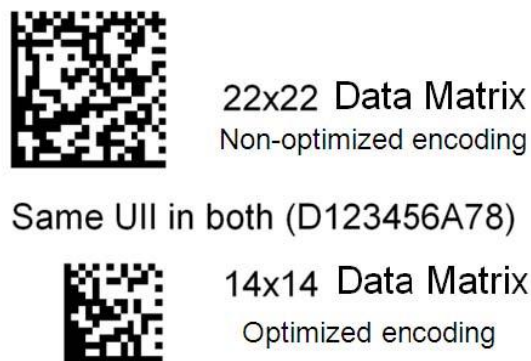
Figure 11. Minimizing Cell Count Through Optimized Encoding
