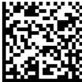
Figure 1. ECC200 Data Matrix Symbol
