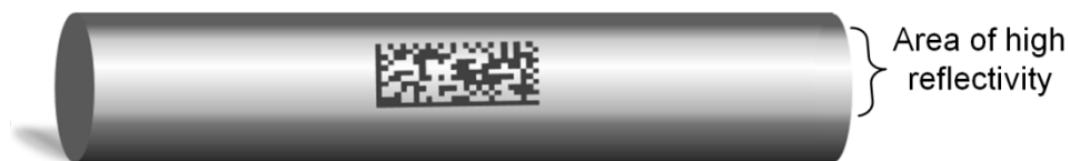
Figure 5. Proper Placement of Data Matrix Symbols on a Curved Surface
