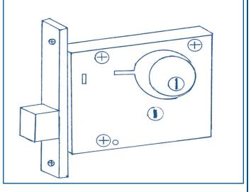
The Federal explosives regulations at 27 CFR Part 555, do not define the term "mortise lock." However, a mortise lock is generally installed in a hollowed-out (or mortised) cavity within the side of a door—with the housing of the lock contained in the door itself—and is actuated by a keyed cylinder on the front of the door.
