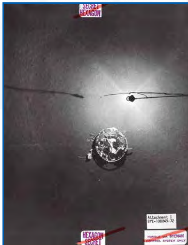
Figure 8: Photograph of the sunken bucket's intact upper structure, taken by the USNS De Steiguer search team on 20 October 1971 at 16,400 feet. Credit: CIA
