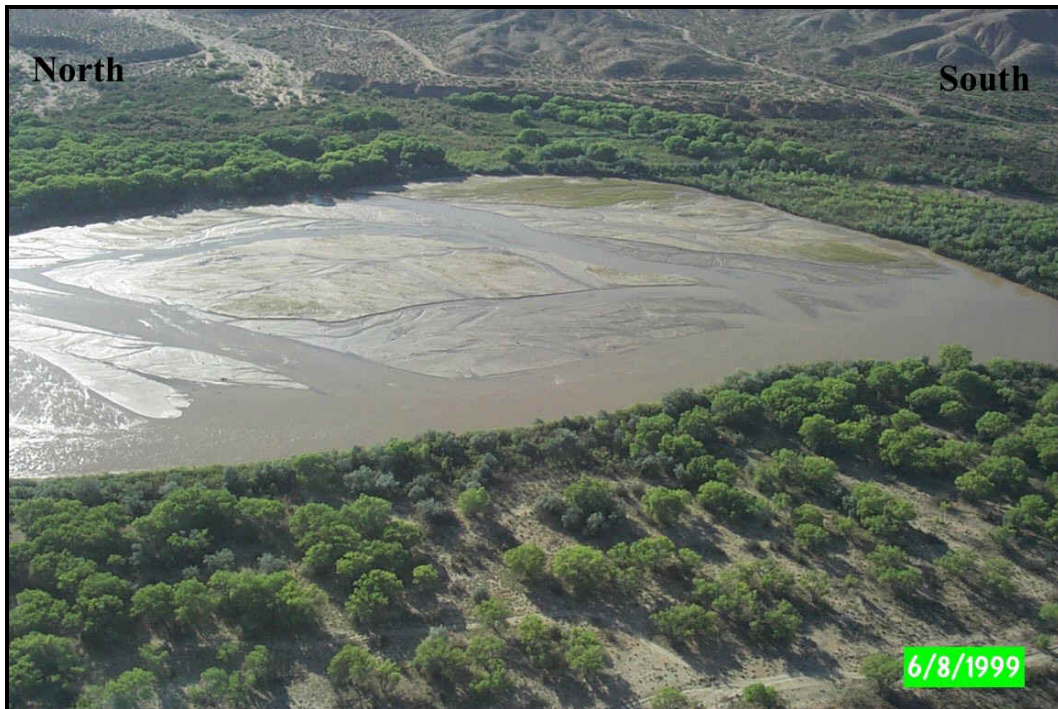
Figure 28. The middle Rio Grande is often characterized by numerous sandbars and a straight channel resulting from the placement of jetty jack fields and levees.
