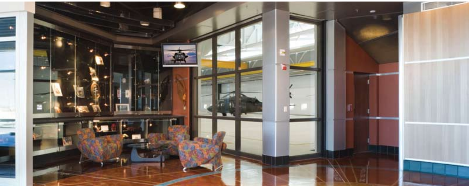
A stained concrete floor with an inlay of flight vectors and compass graphics greets visitors in the lobby.
