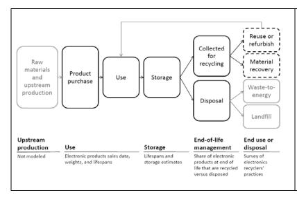
Figure 1: Life-cycle flow chart for electronic products. Solid boxes refer to life cycle stages modeled by the EPA in 2011; dashed and gray boxes refer to stages where information was collected by recycler surveys, or that were not in 2011 modeled. See footnote 2.
