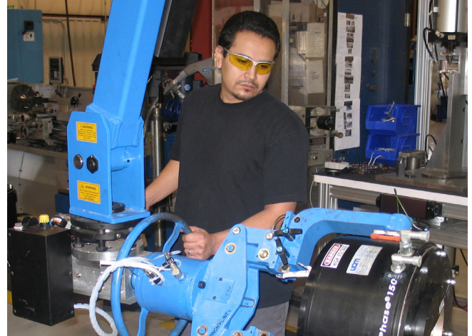
An automotive technician uses robotic equipment to move an electric drive motor. (Photo courtesy of UQM)
