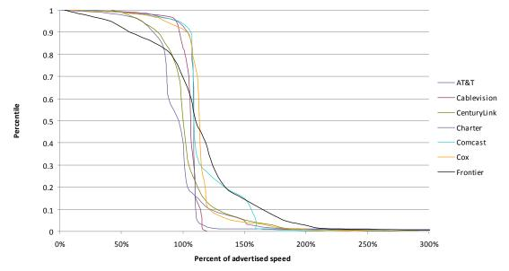
Chart 17.1: Cumulative Distribution of Sustained Upload Speeds as a Percentage of Advertised Speed, by Provider (7 Providers)—April 2012 Test Data
