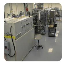
Above: Pulsed electric field (PEF) processing is a non-thermal method of food preservation that uses short bursts of electricity for microbial inactivation and causes minimal or no detrimental effect on food quality attributes. PEF can be used for processing liquid and semi-liquid food products.
