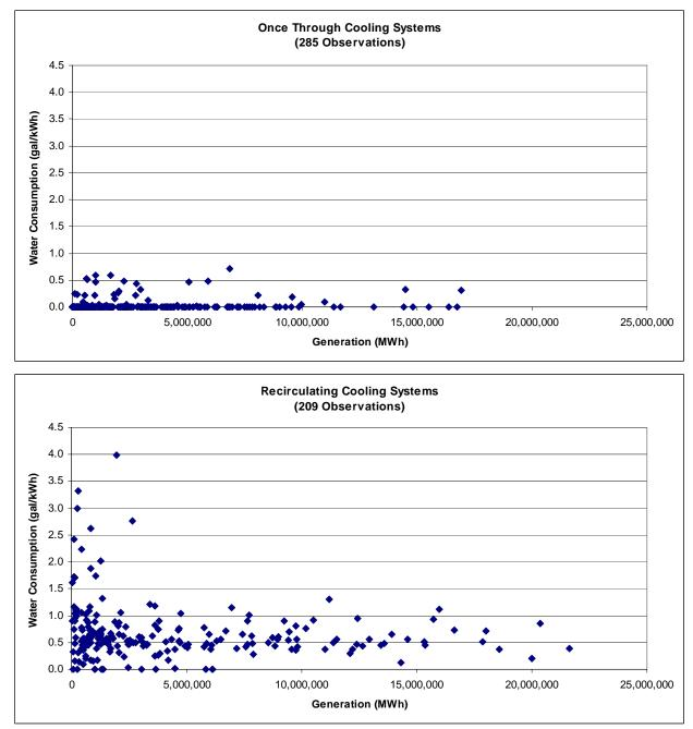
Exhibit 4-3: Water Consumption for Power Plant Cooling Water
