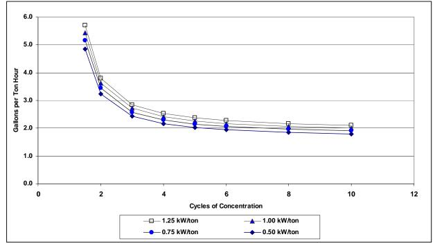
Note: kW/ton of cooling values represent a range of air conditioner efficiencies. More efficient systems (lower kW/ton) require less cooling system water. A "Ton Hour" is one ton of cooling operating for one hour, which is equal to 12,000 Btu of cooling.
