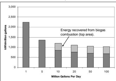
Activated Sludge and Advanced Treatment without Nitrification
