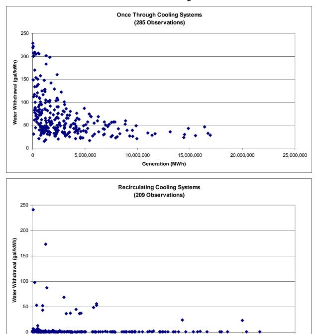
Exhibit 4-2: Water Withdrawal for Power Plant Cooling Water
