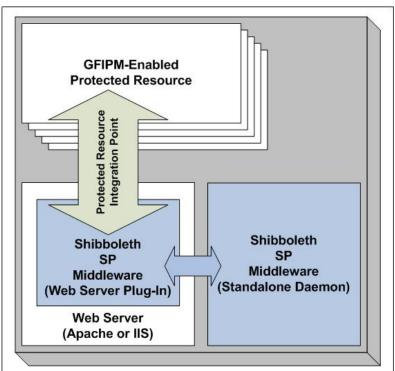
Figure 4: Basic GFIPM Service Provider (SP) Structure
