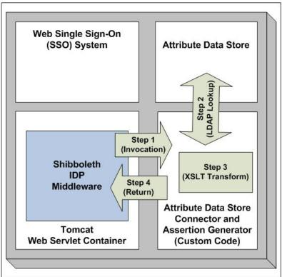
Figure 3: Process of Generating a GFIPM Assertion
