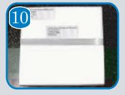
Secure the shipper lid with filamentous shipping tape. Place your return address in the upper left-hand corner of the shipper top and put the CDC Laboratory receiving address in the center.
