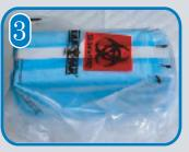
Wrap gridded box in absorbent pad and tape to seal. Seal gridded boxÁnsid^ a Saf-T-PakÁelear inner, leak-proof polybagÁorÁequivalent).
