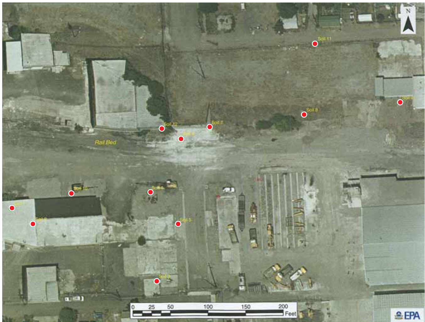
Figure 5 Phase I and II Sample Locations for Soils 1-12. Aerial Photograph Courtesy of Spokane County.
