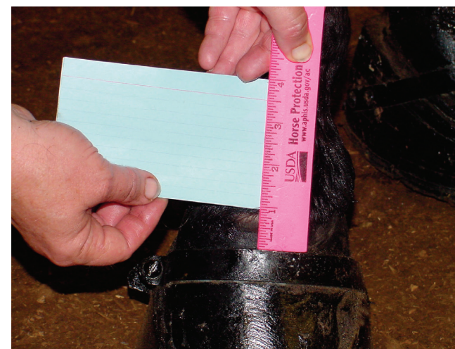
Careful measurements are done to ensure that metal hoof bands are in compliance with the regulations.
