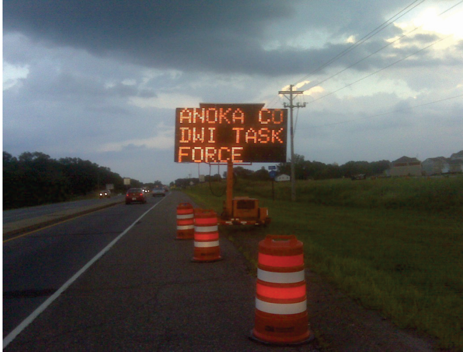
Figure 32. Variable Message Sign
