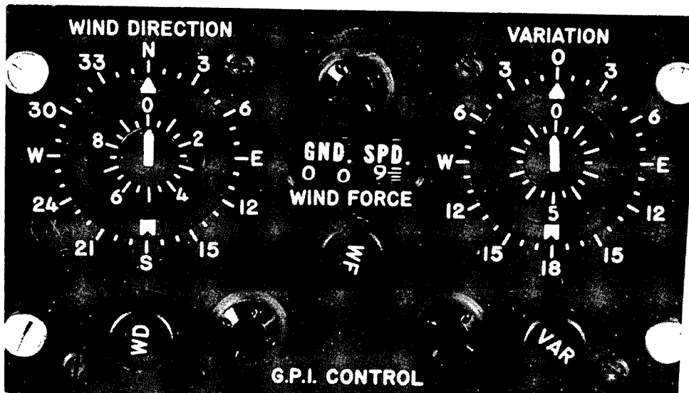
C-1316/ASN-6 RIGHT CONSOLE CONTROL PANEL
