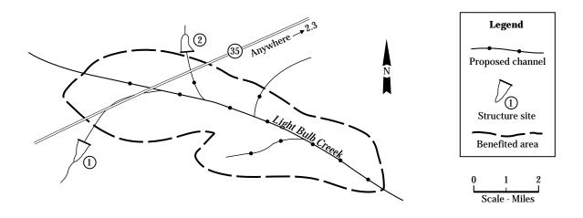
Alternative 2 consists of accelerating land treatment on 1,230 acres of cropland, constructing 2 floodwater retarding structures, and widening and deepening 15.7 miles of channel.
