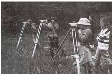
Oregon teachers learn surveying techniques for mapping the boundary and topography of wetland sites.
