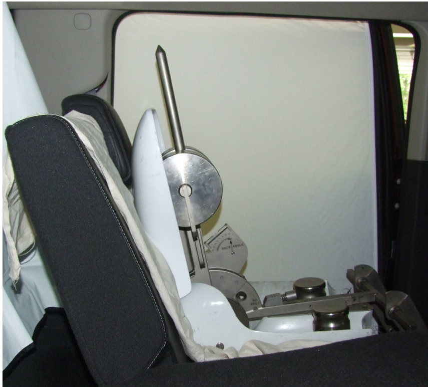
Figure 3. H-point machine as installed in the vehicle (and adjusted per SAE J826) in driver-side outboard 2 nd row seat with OE head restraint in non-use position
