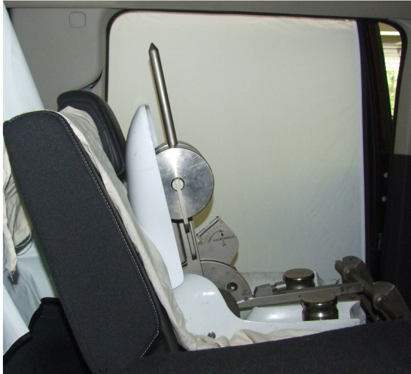
Figure 12. H-point Machine Installed for Measurement of Torso Angle Change.
