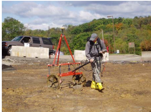
A magnetometer is used to find buried barrels at the NETL-Pittsburgh site.
