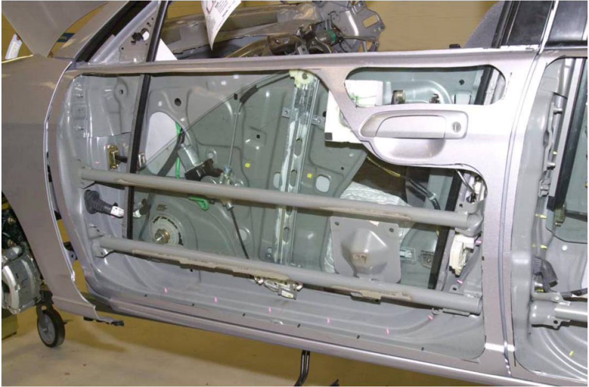
Figure 3-7: Lightweight, tubular front door intrusion beams (2007 Civic)
