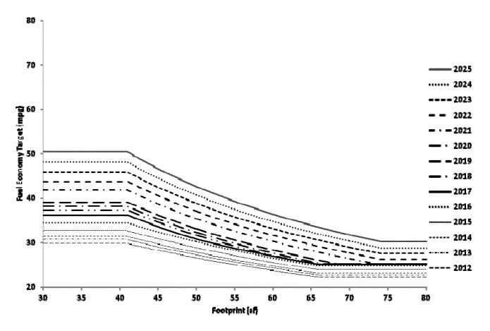
Figure I -2 CAFE Target Curves for Light Trucks
