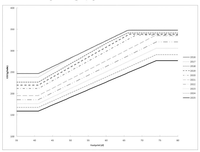
Figure I-4 CO2 (g/mile) Light-Truck Standard Curves
