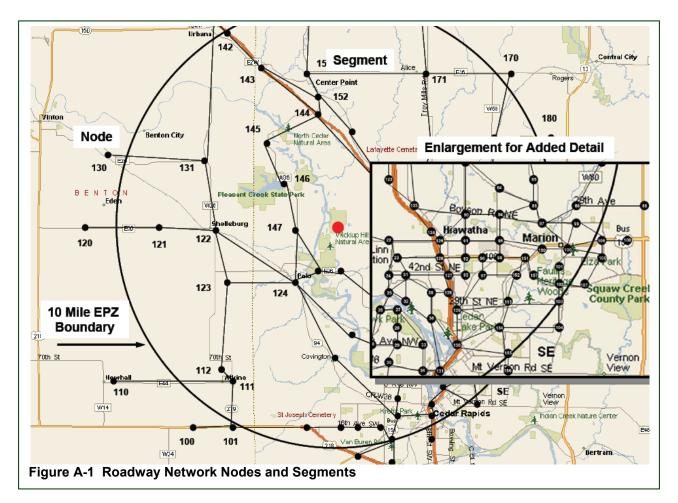
A map of the roadway network should be provided similar to Figure A-1 and should include legible values for nodes and links.
