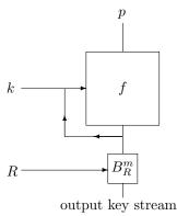
The role of the initialization vector in OFB (the "IV") is taken by the output generation matrix R (the plaintext p may be chosen as a constant), and the initial value of k is the key to our cryptosystem. As for OFB, the IV need not be kept secret, but must be random. The number of bits needed for our IV may at this point seem very large. We shall later discuss ways of significantly reducing the size, while still keeping a provable security. To start with though, we assume it is of "full" size.
