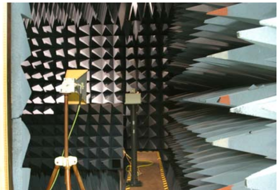
Figure 2: WLAN transmitting node (on pedestal) and receiving antenna (in foreground) in NIST’s anechoic chamber.
