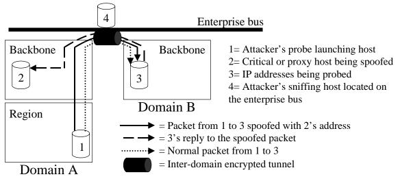
Figure 14.1: Network mapping covert channel attack
