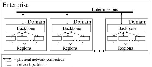
Figure 8.1: Schematic of Network Partitions
