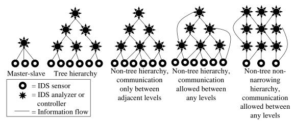
Figure 2.1: Various types of distributed hierarchical IDS architectures
