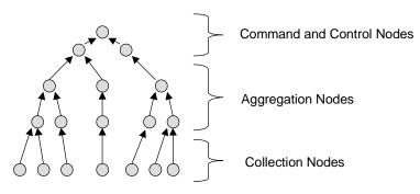
Figure 1: Hierarchical IDS Architecture
