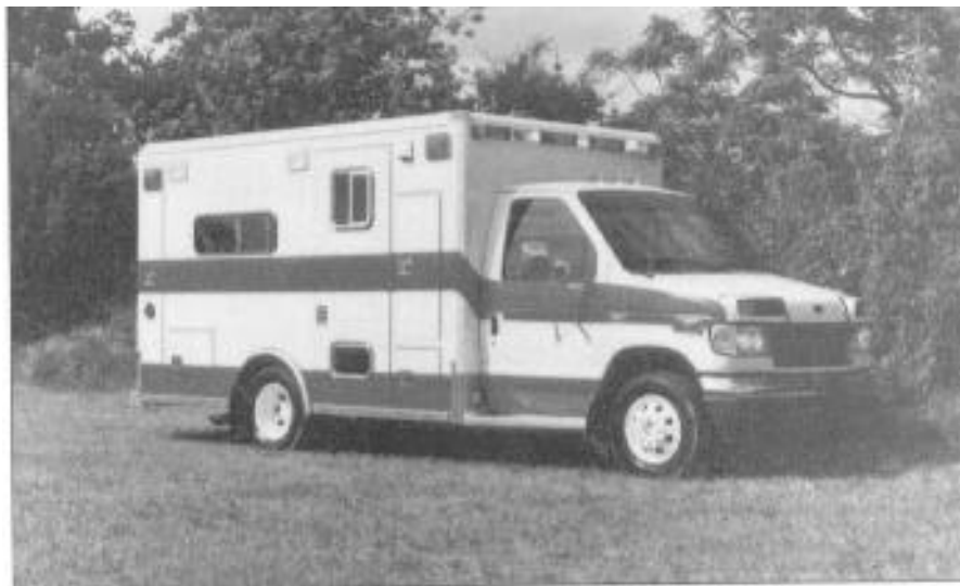
Figure 2-3: A Type III emergency vehicle has a conventional van cab and chassis with a modular patient compartment.
