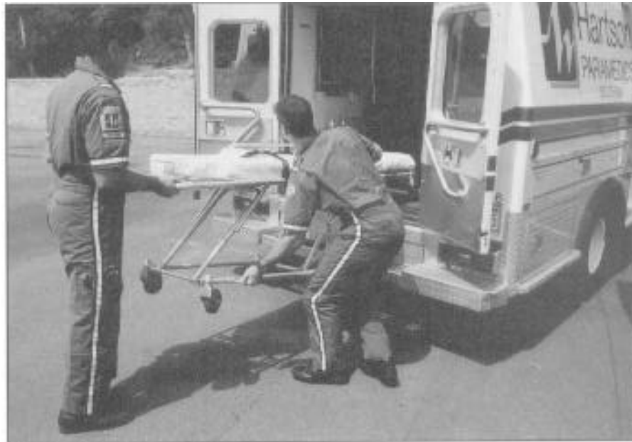
Figure 34: Modern stretcher designs help minimize the exertion needed to lift stretchers into the EMS unit.
