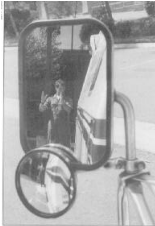
Figure 2-10: Always have a spotter visible in the mirrors when backing an emergency vehicle. Use mutually-understood hand signals. This person is signaling the distance remaining for backing up.
