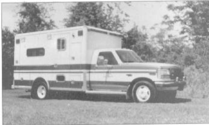
Figure 2-1: A Type I emergency vehicle has a conventional pick-up truck cab and chassis with a modular patient compartment.
