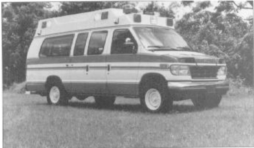
Figure 2-2: A Type II emergency vehicle has a van-type configuration with a raised roof.
