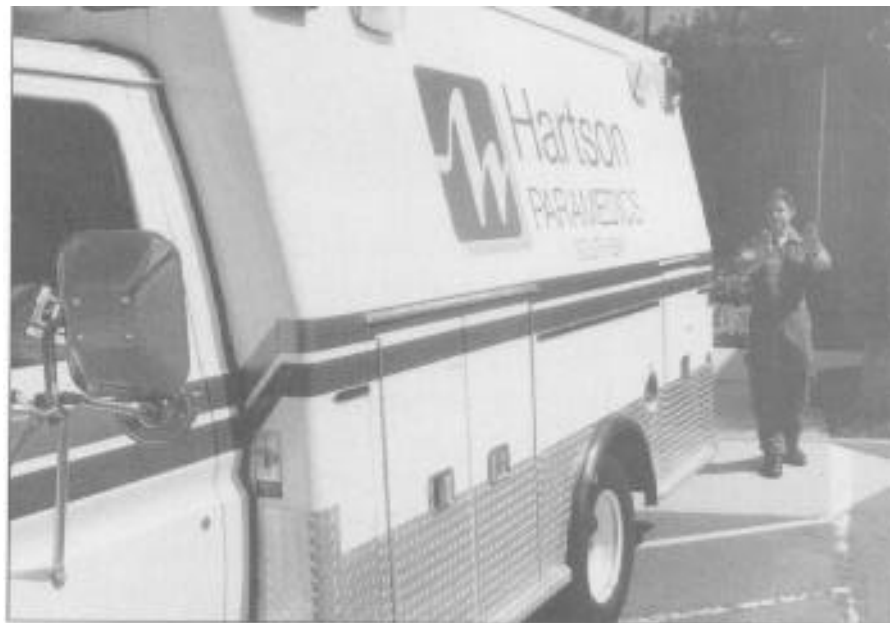
Figure 2-11 : Be sure the spotter stands well away from the backing vehicle. This spotter is signaling the driver to stop.
