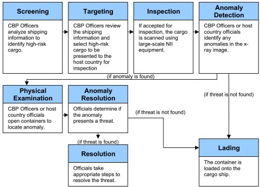
Figure 1: Flowchart of CSI Cargo Screening Process
